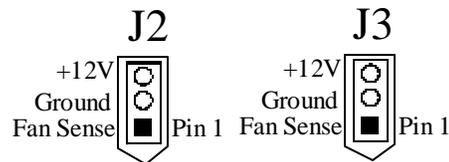
All Pentium Pro CPUs are shipped with a heat sink and a CPU fan. The connector from the CPU fan usually has three leads. The leads are usually yellow, red, and black. Connect the Red lead to Pin 3 +12V. Make sure that you use fans that have 3 leads. The yellow lead should provide a tachometer output to permit the fan speed to be monitored by the onboard server management hardware. If you have to use fans with only 2 leads, connect the red lead to Pin 3.
