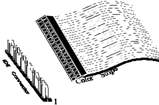
P11 is a 40-pin dual-inline berg that connects an IDE drive to the primary onboard IDE connector. This motherboard supports IDE Modes 0, 1, 2, 3, and 4, IDE prefetch, LBA mode, high capacity drives over 528 MB, 32-bit data transfer, and fast IDE transfer. These IDE features are configured in Peripheral Setup in the WINBIOS Setup utility.
