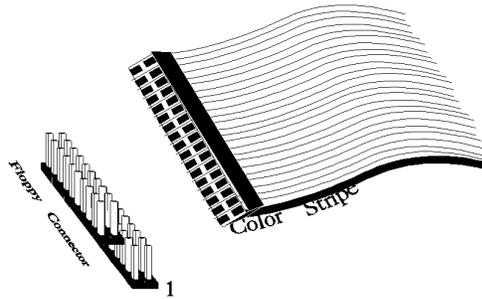
The motherboard supports up to two 720 KB, 1.44 MB, or 2.88 MB 3½" drives and 360 KB and 1.2 MB 5¼" drives. The connecting cable is a 34-pin ribbon connector with two 34-pin edge connectors for attaching the floppy disk drives. There is a small twist in the cable between the floppy connectors. The last connector should be connected to floppy drive A:
