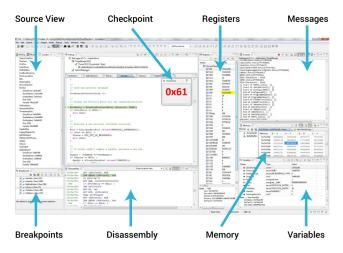
AMI Debug for UEFI is a powerful solution for debugging Unified EFI (UEFI) projects, offering source-level debugging without the need for an expensive in-circuit emulator (ICE). Using standard RS-232, USB 2.0 cables or the AMI Debug Rx device and USB 3.0 Debug Cable, developers have access to source-level debugging and control the debug target hardware through a GUI application for Microsoft Windows.
